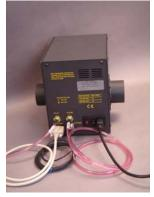
14. If applicable, connect CO2 tube to push to release connector marked "CO2 Port 1" on the back of the chamber.
